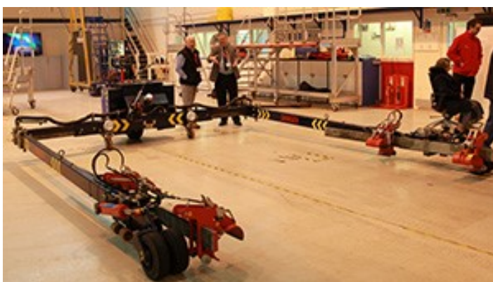
Helicopter Moving equipment
